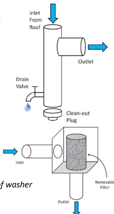
*Figure 2. A box-type roof washer with removable filter.*
